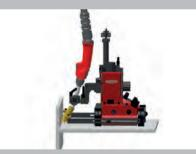
/ Welding fillet welds on horizontal components
