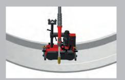
/ Welding butt welds on concave components
