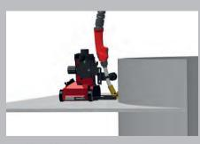
/ Welding fillet welds on convex components
