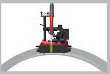
/ Welding butt welds on convex components
