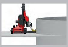
/ Welding fillet welds on convex components
